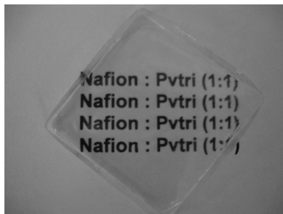
Fig. 2. Transparent and thin film of Nafion–P(VTri) 11 blend membrane.
